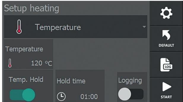
By pressing “**Hold Time**” you can adjust the hold temp duration of the workpiece. The time is entered in mm:ss and can be set between 00:01 and 99:00.
