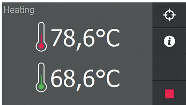
Once the set temperature, in this example 80°C, is reached for the first time, a timer will appear at the bottom of the screen, indicating the remaining time the workpiece is kept at the set temperature.
