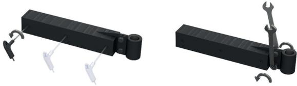
3. Loosen the socket screws and the bolts on the hinge bushing by about half a turn.
