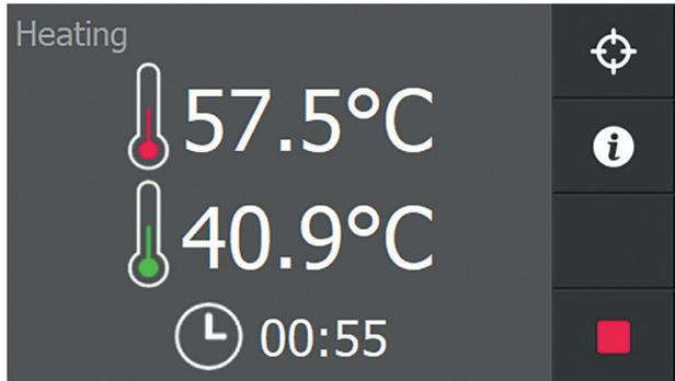
By pressing the info button **i**, the heating process is displayed graphically. Pressing info again displays additional information from the process.
