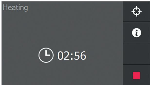
Only when sensors are connected, the heating process is displayed graphically by pressing the info button **i**. Pressing info again displays additional information from the process.
