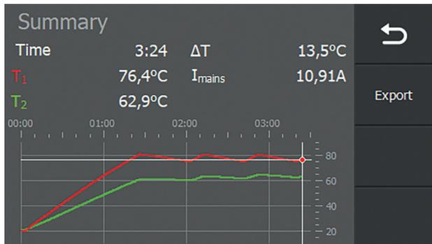
**11.3  $\Delta T$  functionality** This functionality is used if the temperatures in a workpiece must not differ too much in order to avoid stresses in the material. The functionality is also used for bearings when the temperatures of the inner ring and outer ring must not differ too much. If necessary, ask the supplier of the workpiece what the maximum temperature difference in the workpiece may be.
