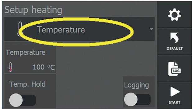
The various heating modes can be selected by tapping the current mode on the settings screen.
