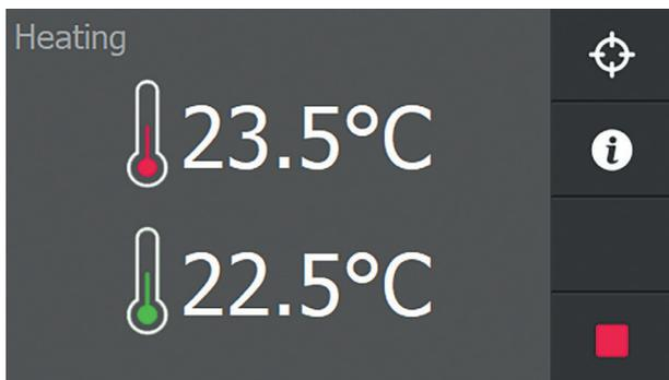
Pressing this button during heating allows the desired temperature or time (target) to be adjusted up or down without having to stop the process. By pressing “**Target**”, a screen with the current setting and current value is displayed first.
