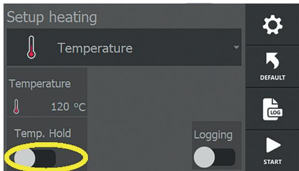
This functionality enables a workpiece to be held at a set temperature once that temperature has been reached. Maintaining the temperature of a workpiece follows a certain switching hysteresis (T hold hysteresis), which can be set in the system settings as described in section 6.4. The temperature set here is the temperature to which a workpiece may drop before the heater switches on again automatically.
